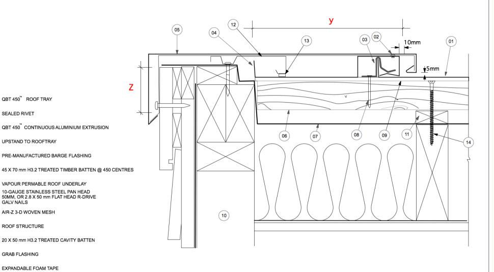
(10) ROOF STRUCTURE 11 20 X 50 mm H3.2 TREATED CAVITY BATTEN
